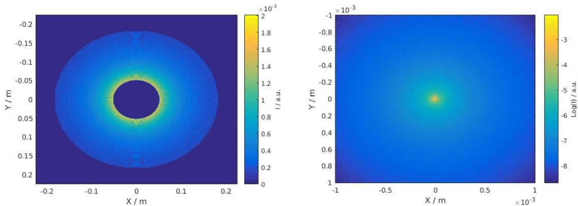
Figure 4. Transversal intensity distribution for a NuSTAR-like telescope, with conical, concentric shells with radii ranging from  $\approx 5.5\text{mm}$  to  $\approx 19\text{mm}$ . Right: Shortly after the optic, Left: At the focal point. For clarity we plot  $\log(I)$
