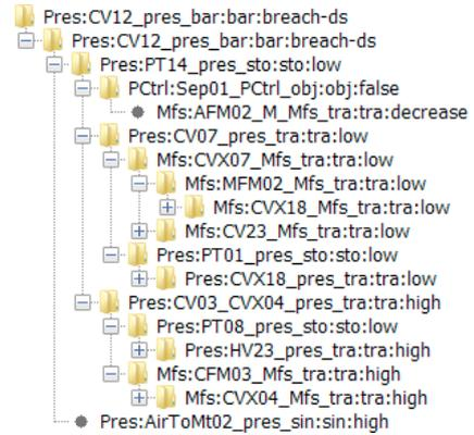
Fig. 8. Consequence paths for the CV12 breach downstream
