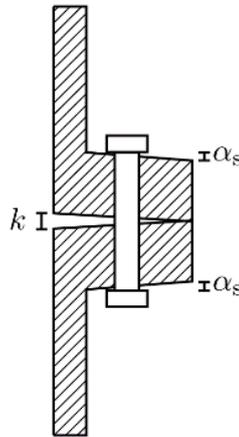
**Figure 5.** Specification of flange tolerances. Figure from [9].
