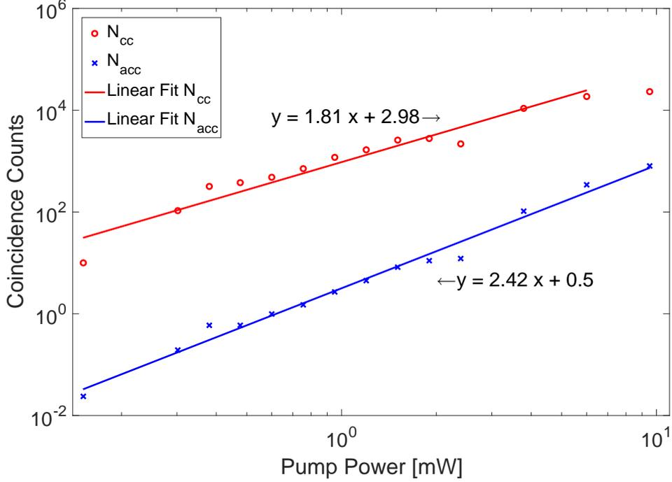
**Fig. 3.** Coincidence counts and accidental coincidence counts showing approximately quadratic behavior. All points are obtained from 600 s measurements. In the linear fits  $y = \log_{10}(N_{cc})$  and  $x = \log_{10}(P_p/\text{mW})$ .
