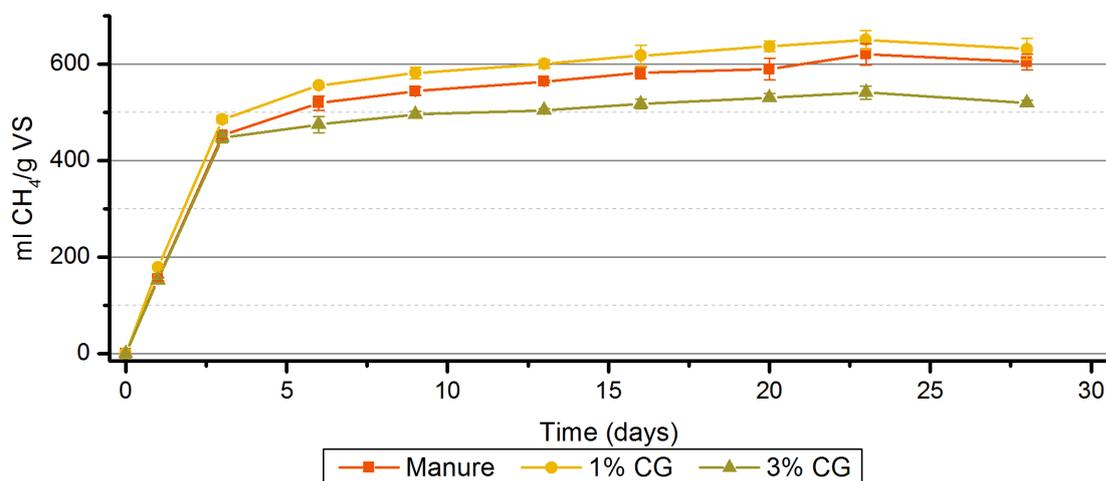
**Figure 3.** Cumulative CH<sub>4</sub> yields of second set of BMPs of manure, 99% of manure and 1% CG (1% CG), and 97% manure and 3% CG (3% CG).
