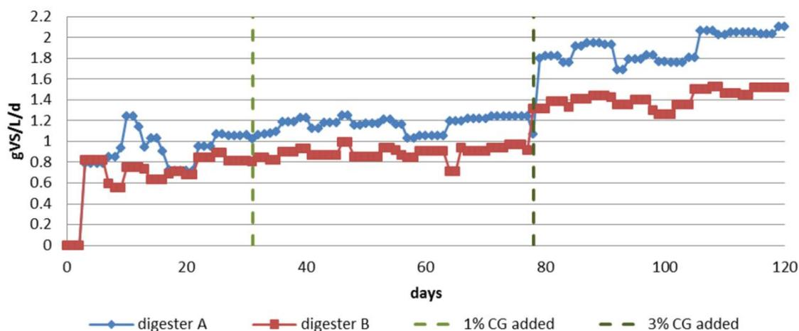
**Figure 5.** Organic Loading Rate of digesters A and B during the entire course of experiments.
