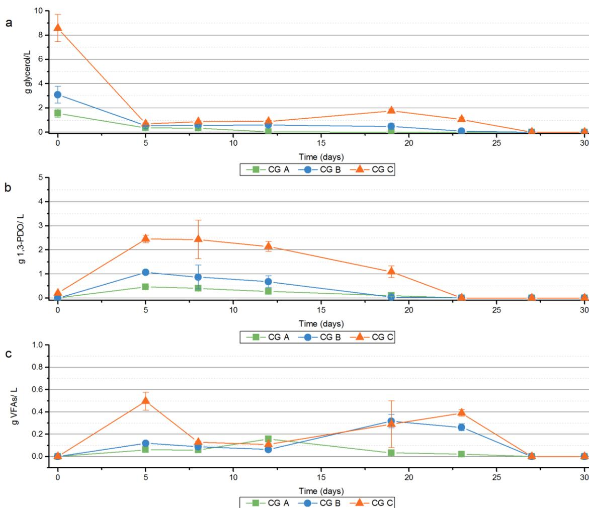
**Figure 2.** Evolution of (a) glycerol concentration, (b) 1,3-PDO concentration and (c) VFA concentration in BMP tests of CG at different organic loadings. CG A, B and C correspond to I:S ratio on a VS basis of 4:1, 2:1 and 1:1 respectively.
