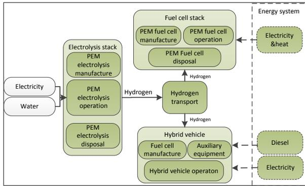
Fig. 1. System boundary of hydrogen production and application
