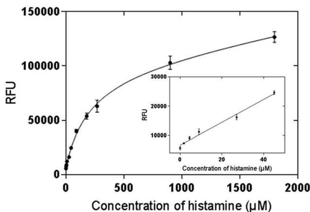
Fig. 6 Saturation curve and calibration curve of histamine nanoMIP-based OPA fluorometric assay. Error bars were for experiments performed in duplicates. The  $R^2$  value of calibration curve was 0.992.
