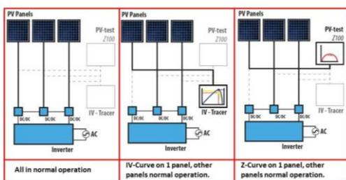
Fig. 1. Working principle of the field test.
