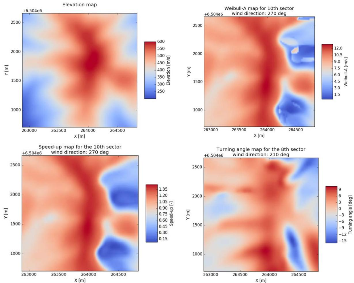
**Figure 2.** Terrain and wind resource information for a complex terrain site: (up-left) elevation; (up-right) Weibull-A parameter; (down-left) speed-up factor; (down-right) turning angle.
