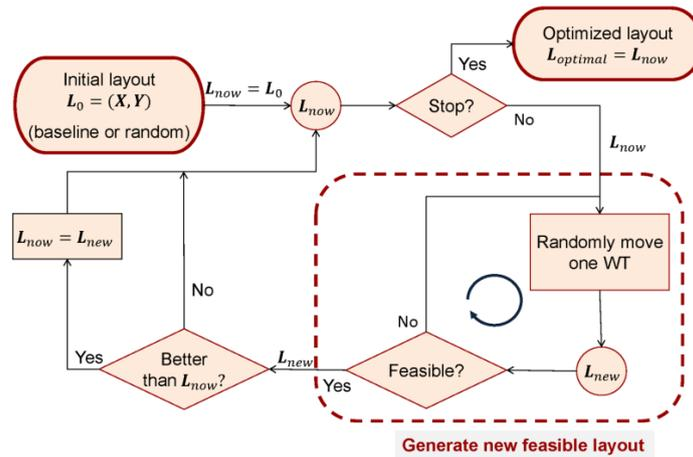
**Figure 4.** Flowchart of the Random Search algorithm for layout optimization
