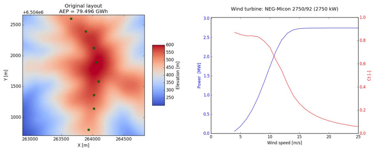
**Figure 5.** A small wind farm in complex terrain: (left) the original layout; (right) WT characteristics
