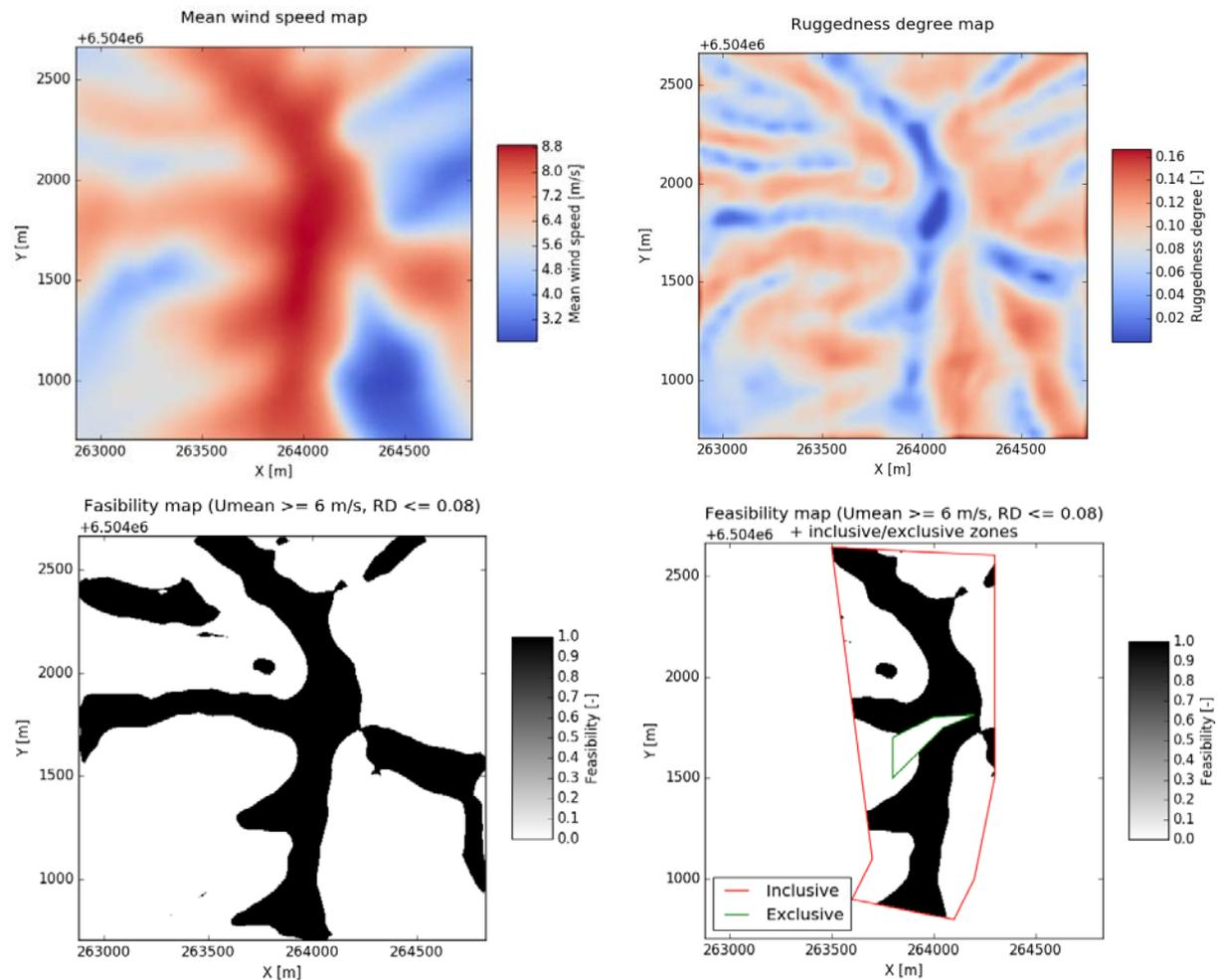
**Figure 3.** Constraint modelling of FarmOpt: (up-left) map of mean wind speed; (up-right) map of ruggedness degree; (down-left) constraints on minimal mean wind speed and maximal ruggedness degree; (down-right) adding constraints on inclusive zone and exclusive zone.
