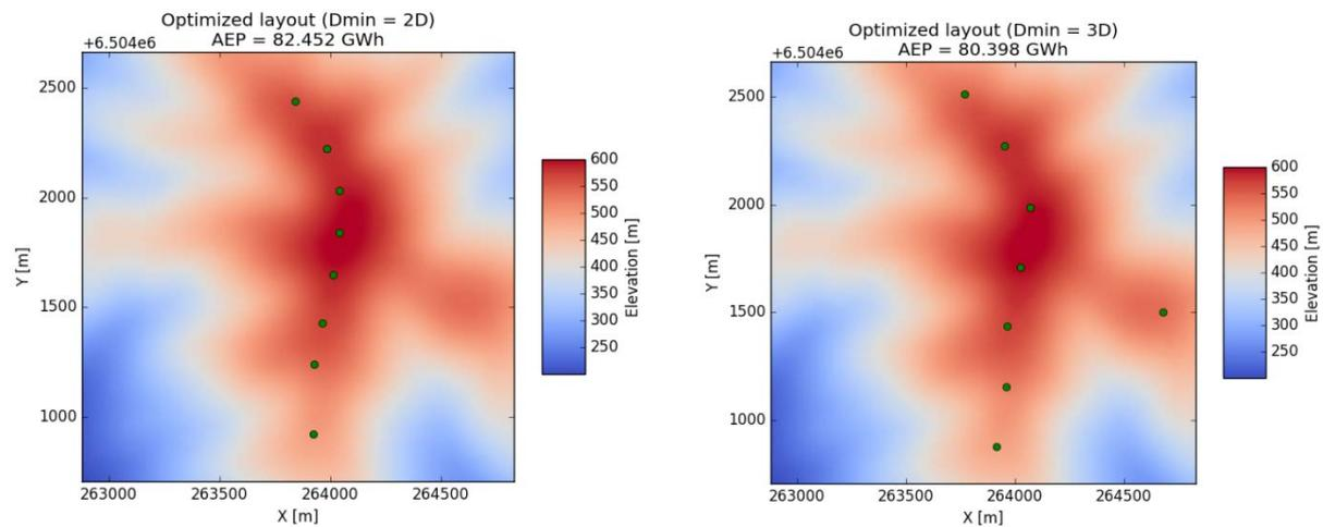
**Figure 6.** Optimized layouts with different minimal distance requirements using 1000 evaluations
