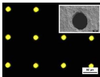
Figure 2. Microscope dark field image of a  $2 \times 2 \text{cm}$  2D holes grating made in  $50 \mu\text{m}$  thick tungsten substrate using laser ablation. Insert: SEM image of  $17 \pm 0.5 \mu\text{m}$   $\varnothing$  holes. Scale  $5 \mu\text{m}$ .
