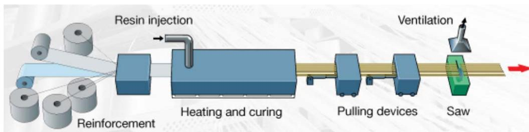
Figure 1: Sketch of the RIP process (courtesy of Fiberline).
