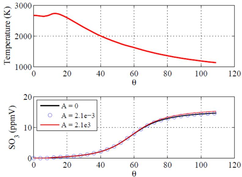
Figure 5: Mean temperature and overall  $\text{SO}_3$  concentration of the burned gas during combustion and expansion until the exhaust valve opens. The figure shows the effect of a factor 1000 change in the pre-exponential factor  $A$  for the catalytic vanadium reaction (R1).
