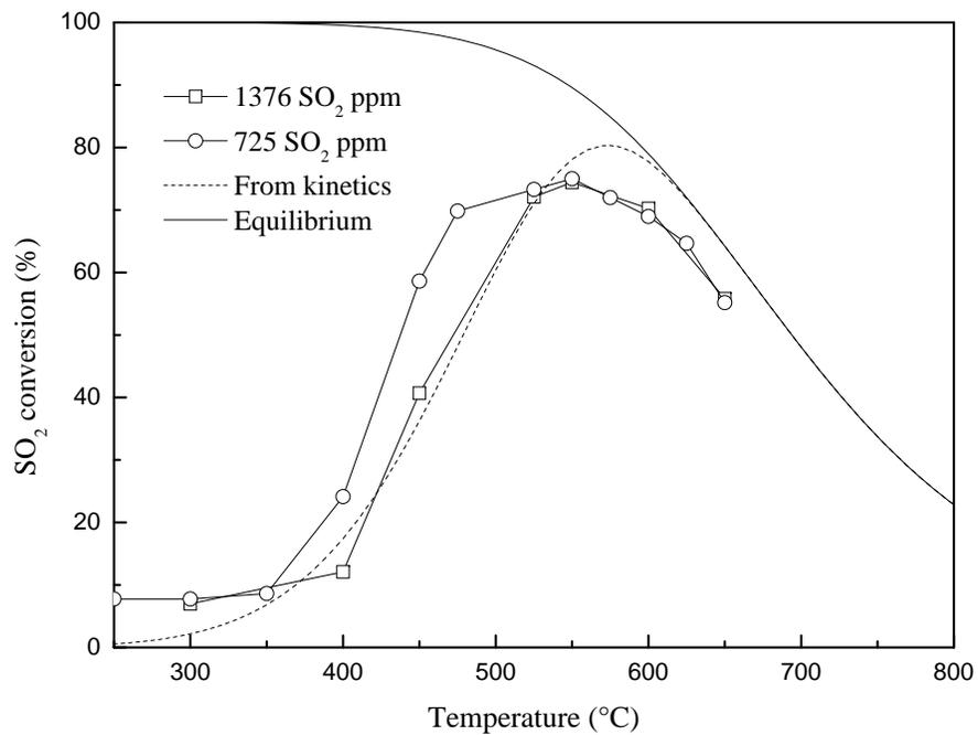
Figure 2: Conversion of SO<sub>2</sub> for two different initial concentrations of SO<sub>2</sub> and same catalyst (V/Na = 7.9). Comparison between experimental results and predictions with the kinetic model are also shown.
