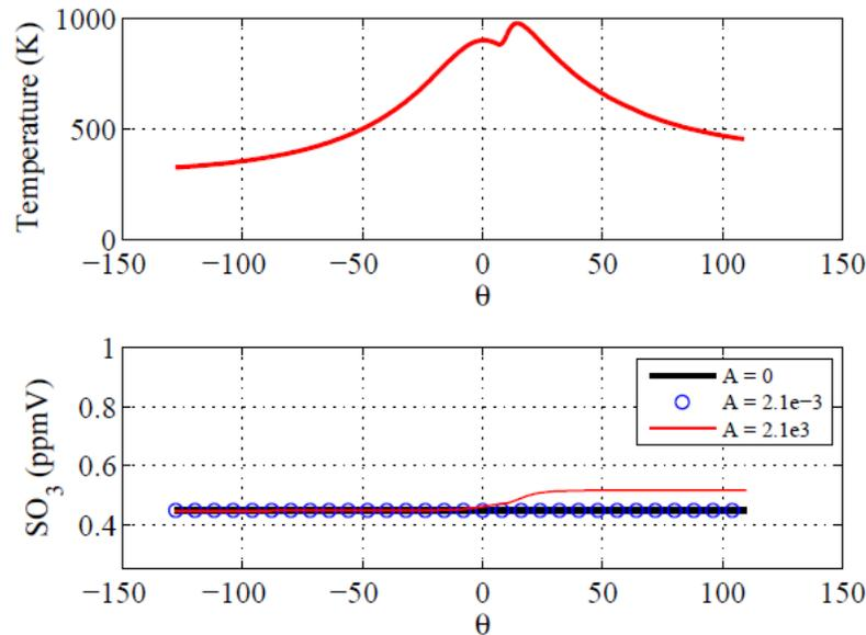
Figure 7: Fresh gas temperature and catalytic  $\text{SO}_3$  formation in the fresh gas over the engine cycle. The figure shows the effect of a factor 1000 change in the pre-exponential factor  $A$  for the catalytic vanadium reaction (R1).
