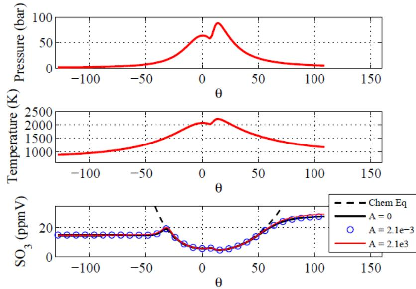
Figure 6: Cylinder gas pressure, residual gas temperature and catalytic  $\text{SO}_3$  formation in the residual gas over the engine cycle. The figure shows the effect of a factor 1000 change in the pre-exponential factor  $A$  for the catalytic vanadium reaction (R1).
