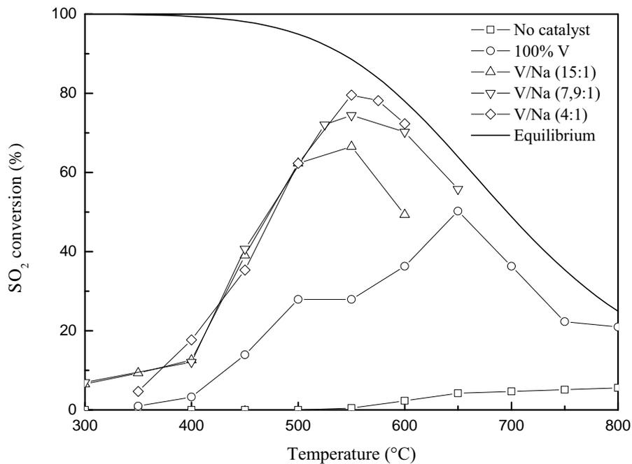
Figure 1: The effect of catalyst composition and temperature on the oxidation of SO<sub>2</sub> in the fixed-bed reactor. Results are shown for experiments with an empty reactor, with pure vanadium, and with particles with V/Na ratios in the range 4-15 (mass based). Flow rate: 157.4 mL min<sup>-1</sup> (25°C, 1 atm); 1376 ppm SO<sub>2</sub>, 14% O<sub>2</sub>, 2.6% H<sub>2</sub>O, balanced with N<sub>2</sub>.
