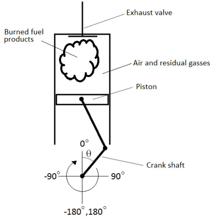
Figure 4: Sketch of a two-stroke engine cylinder
