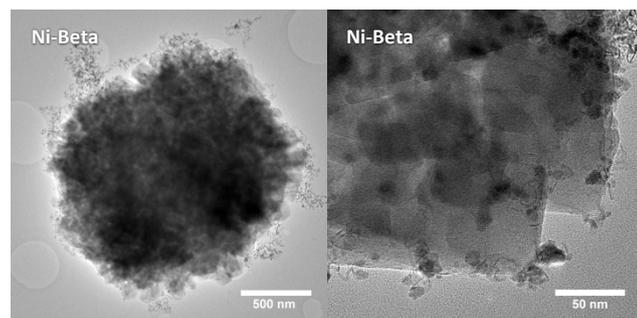
Fig. 5. TEM images of mesoporous Beta-type materials.
