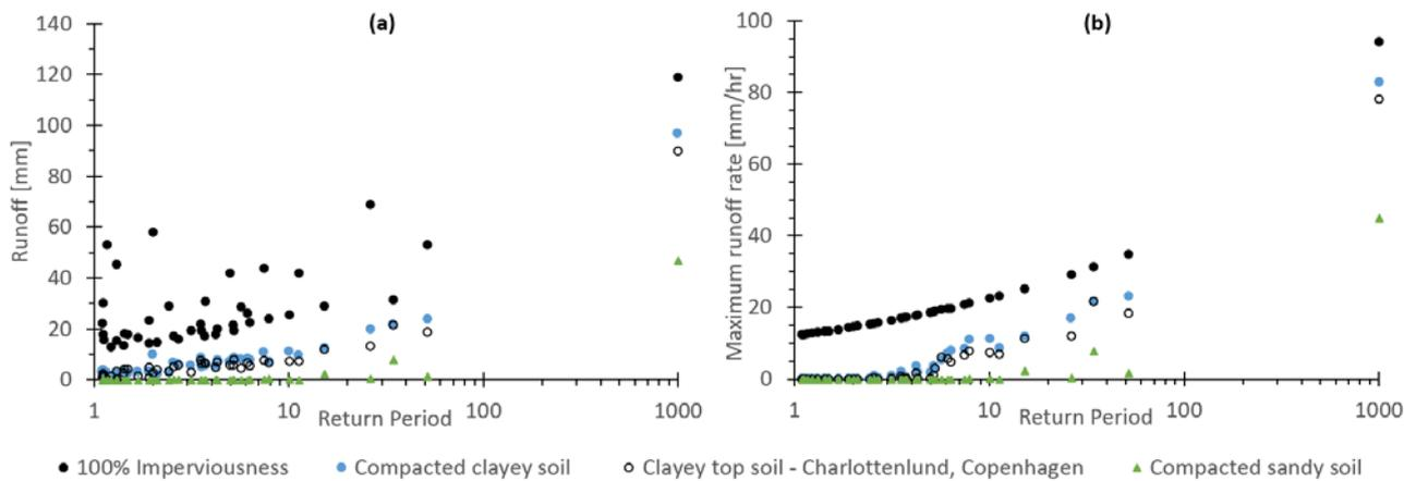
**Fig. 3.** (a) Simulated total runoff depth for historical rain events with return periods based on the maximum hourly rain intensity. There is no simulated runoff from non-compacted sandy soils. (b) Simulated maximum hourly runoff rate for the same historical rain events.
