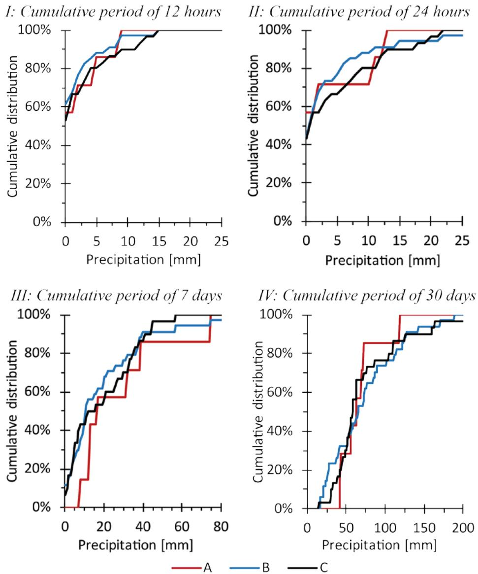
**Fig. 1.** Percentage of rain events where accumulated precipitation prior to the event is less than a given threshold. Shown for different durations before the event (subfigures I-IV) and for events with different return periods  $T$  (coloured lines, A (red):  $T > 10$  years, B (blue):  $T = 1-10$  years, C (black):  $T = 0.5-1$  years).
