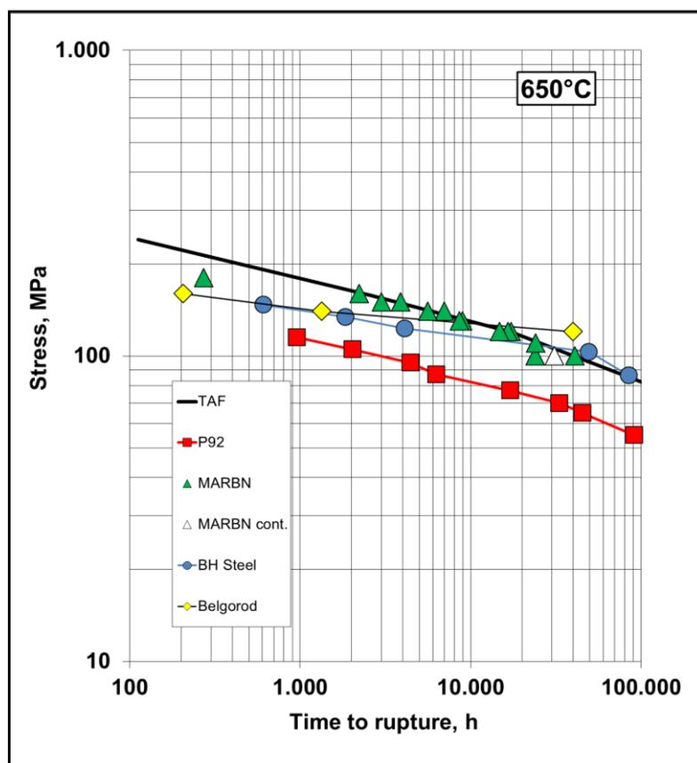
Figure 2. Creep rupture strength of new 9-10%Cr steels.
