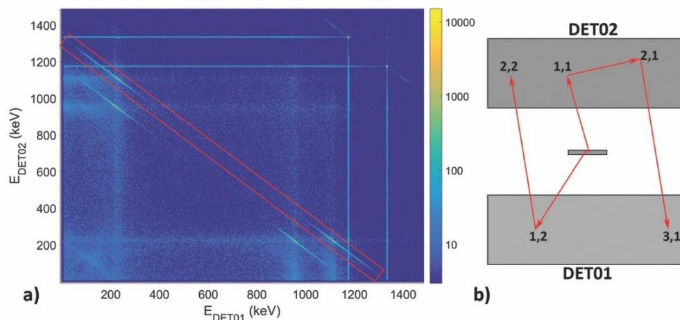
Figure 1. a) 2D coincidence spectrum of  $^{60}\text{Co}$  point source. Coincidences that are coming from a single 1332.5 keV gamma line depositing its energy in both detectors are shown in red square. b) Example of two gamma ray traces leading to diagonal lines in the left.
