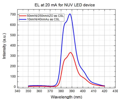
Fig. 1. EL of LEDs with different CSLs
