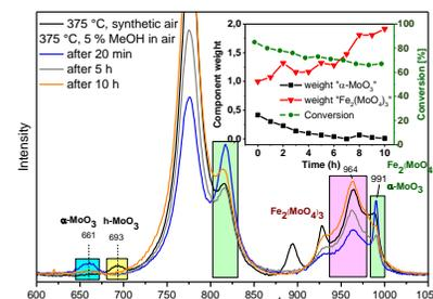
**Figure 2.** *In situ* Raman spectra after 20 min, 5 h and 10 h on stream during methanol oxidation. Inset: Corresponding MeOH conversion and weight parameters representative for α-MoO<sub>3</sub> and Fe<sub>2</sub>(MoO<sub>4</sub>)<sub>3</sub>.
