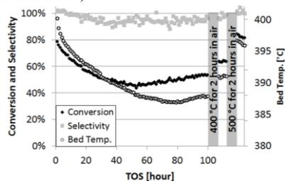
**Figure 1.** MeOH conversion, formaldehyde selectivity and catalyst bed temp. in the fixed bed reactor. Operating conditions: 25 mg catalyst diluted in 170 mg SiC, ~157.5 NmL/min gas feed: 10 % O<sub>2</sub>, ~5 % MeOH in N<sub>2</sub>. Other products: DME and small amounts of CO and CO<sub>2</sub> (< 1 C-mol.%).
