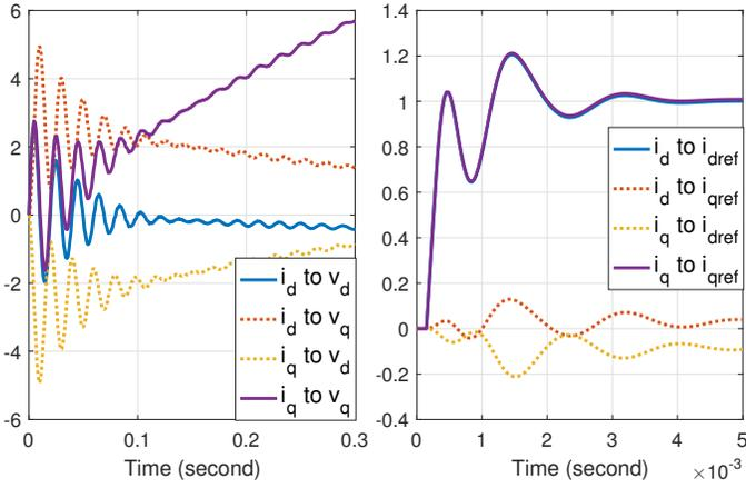
Fig. 7: Step response of  $J_{CC}$  (left) and closed-loop model of CC (right) for converter one. The magnitudes are given in per unit.
