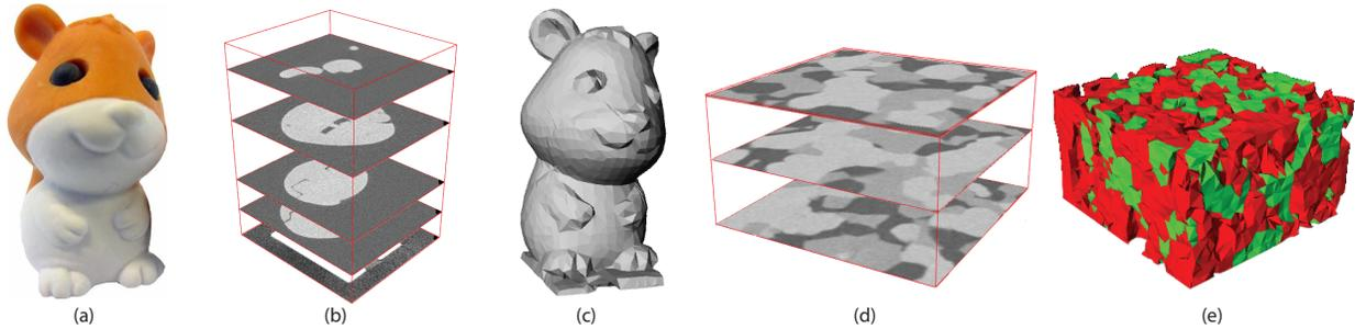
**Figure 1: (a) A ceramic hamster toy used for testing. (b) CT scan of the hamster. (c) Segmentation of the hamster. (d) Scan of fuel cells. (e) Segmentation of the fuel cells scan to three phases: Red, green and the air (transparent).**
