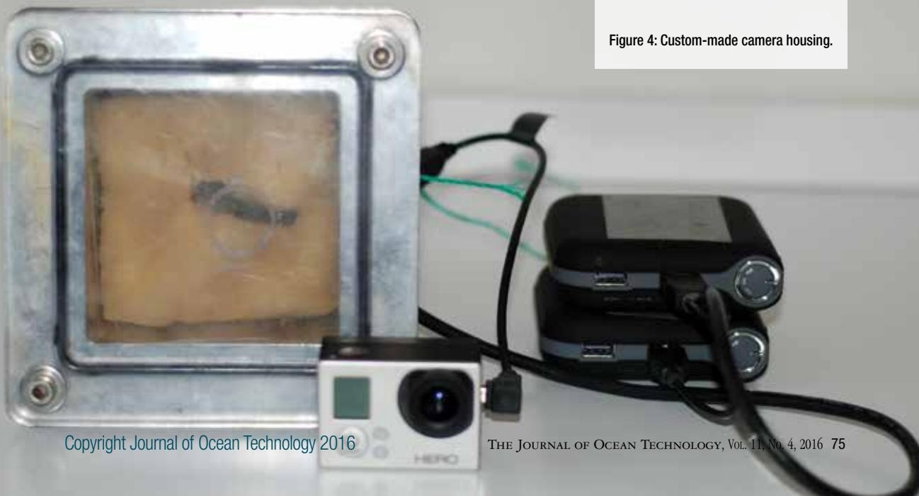
Figure 4: Custom-made camera housing.
