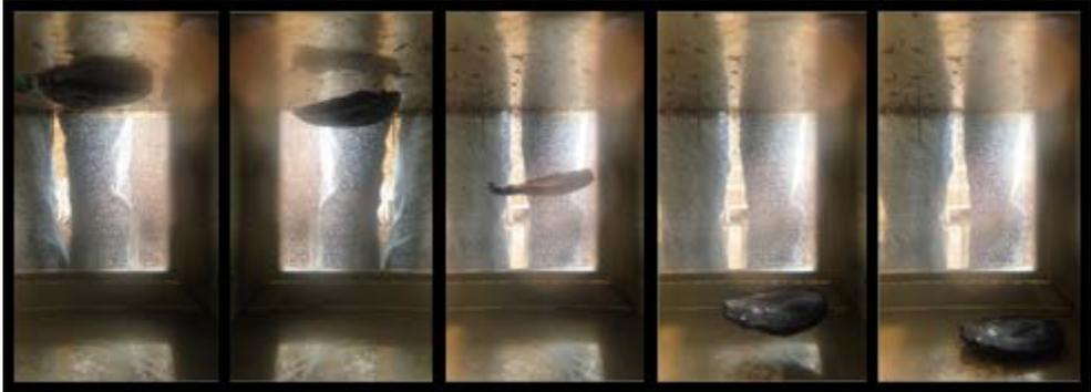
*Figure 1: Illustration of the sinking of the residue after flame extinction for the burning of IF30, 40 mm initial thickness. Each picture illustrates approximately a time interval of 2 s.*
