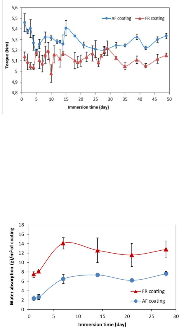
Figure 2: The average torque values of daily measurements for AF coating and FR coating during the entire immersion period at a temperature of  $20 \pm 2$  °C and a speed of  $400 \pm 1$  RPM (left). Water absorption of AF and FR coating from standard WAT as a function of immersion time (right). Error bars for daily measurements based on three replicates are also shown in the plots.
