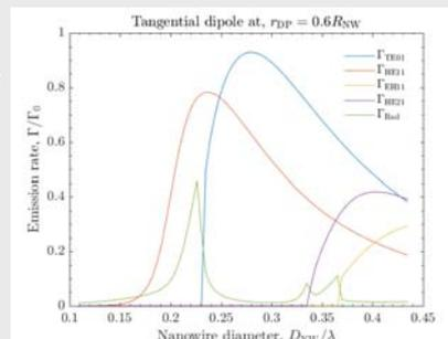
Figure 5: Spontaneous emission rate for a dipole in a Nanowire placed  $0.6 R_{NW}$  off axis.
