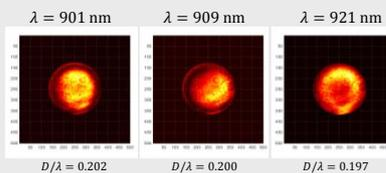
Figure 3: Measured far-fields for three different quantum dots.
