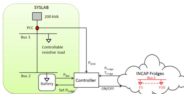
Fig. 1. SYSLAB experimental setup.
