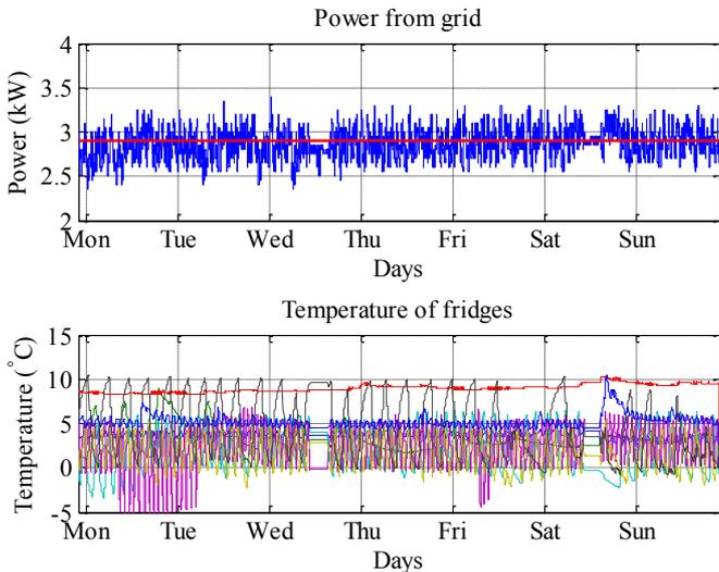
Fig. 5. Power from grid and temperature of fridges in different colors without fridge control. (1 second sampling)
