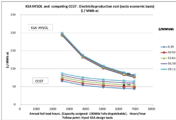
**Fig. 4 Electricity production costs for Combined Cycle Gas Turbine (CCGT) and KSA HYSOL configuration, as function of load factor and NG price. Assumed: CO<sub>2</sub> costs = 40 \$/tonCO<sub>2</sub>, R=4 %p.a., Lifetime=25 years. Unit: \$/MWh el.**
