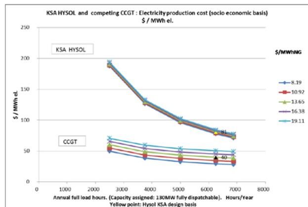
Fig. 3 Electricity production costs for Combined Cycle Gas Turbine (CCGT) and KSA HYSOL configuration, as function of load factor and NG price. Assumed: CO<sub>2</sub> costs = 0 \$/tonCO<sub>2</sub>, R=4 %p.a., Lifetime=25 years. Unit: \$/MWh el.
