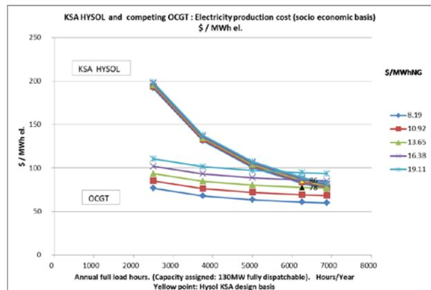
Fig. 2 Electricity production costs for Open Cycle Gas Turbine (OCGT) and KSA HYSOL configuration, as function of load factor and NG price. Assumed: CO<sub>2</sub> costs = 40 \$/tonCO<sub>2</sub>, R=4 %p.a., Lifetime=25 years. Unit: \$/MWh el.
