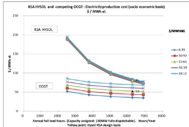
Fig. 1 Electricity production costs for Open Cycle Gas Turbine (OCGT) and KSA HYSOL configuration, as function of load factor and NG price. Assumed: CO<sub>2</sub> costs = 0 \$/ton CO<sub>2</sub>, R=4 %p.a., Lifetime=25 years. Unit: \$/MWh el
