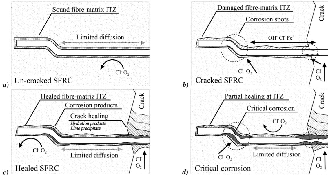
**Fig. 4.** Structure and corrosion mechanisms on: a) Un-cracked SFRC; b) Cracked SFRC at an early stage; c) Cracked SFRC after autogenous healing; d) Cracked SFRC with critical corrosion on fibres.
