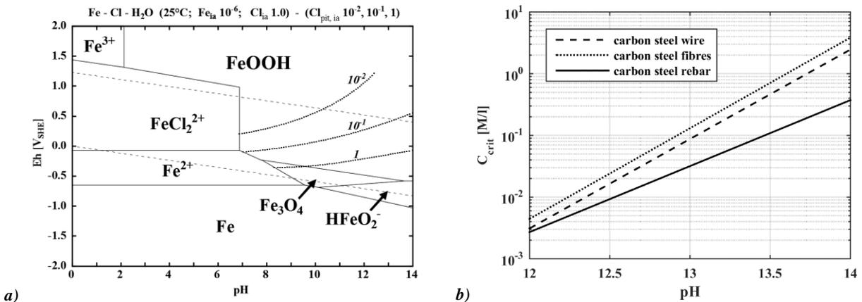
**Fig. 1.** Critical chloride concentrations for pitting corrosion on: a) Potential-pH diagram with superimposed pitting-potential curves for conventional steel, after Küter et al. (2006); b) critical chloride content at different pH values for conventional steel and steel fibres, after Dauberschmidt (2006, 2014).
