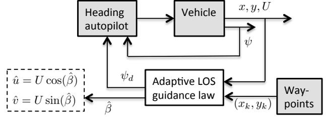
Fig. 2. The adaptive integral LOS guidance law as reference generator to a commercial autopilot system. The estimated sideslip angle  $\hat{\beta}$  also gives estimates  $\hat{u}$  and  $\hat{v}$  of the surge and sway velocities, respectively.
