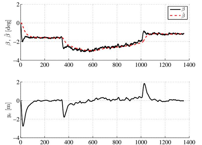
Fig. 7. Curved-path path following while being subject to a stochastic current. The plots show the estimated sideslip angle  $\hat{\beta}$  in comparison to the true  $\beta$ , and the cross-track error  $y_e$ .
