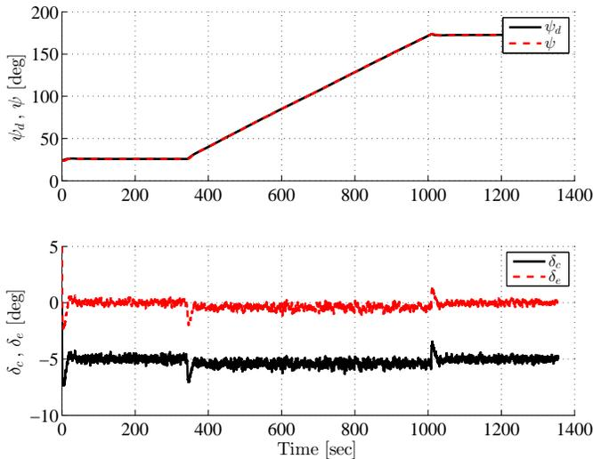
Fig. 8. Curved-path path following while being subject to a stochastic current. The plots show the desired and actual heading angle  $\psi_d$  and  $\psi$ , and the commanded and executed rudder angle  $\delta_c$  and  $\delta_e$ .
