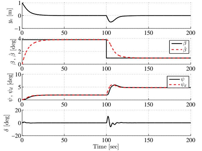
Fig. 3. Straight-line path following. The plots show the cross-track error  $y_e$ , estimated sideslip angle  $\hat{\beta}$ , desired and actual heading angle  $\psi_d$  and  $\psi$ , respectively, and rudder angle  $\delta$ .
