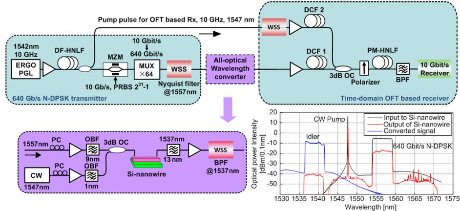
Fig. 2, Experimental setup and the optical spectra before and after the Si-nanowire
