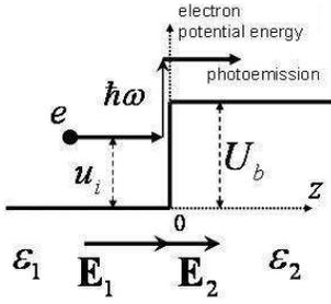
Figure 2. Photoelectron emission from metal: an electron with energy  $u_i$  absorbs a photon with energy  $\hbar\omega$  during collision with the potential barrier  $U_b$  at the metal boundary, overcomes the barrier and leaves the metal.
