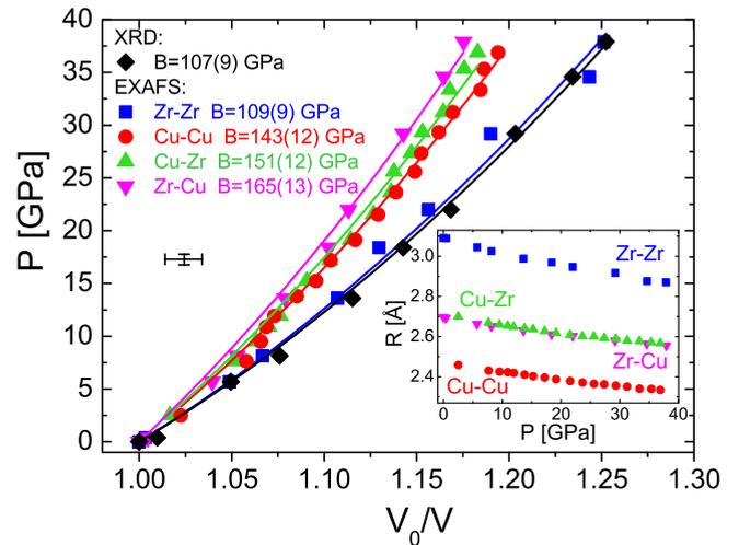
FIG. 3. The results of Birch-Murnaghan EOS fitting to XRD and EXAFS data (cross indicates error bars). The evolution of interatomic distances derived from EXAFS fitting is shown in the inset. The error bars of  $R$  are smaller than symbols.
