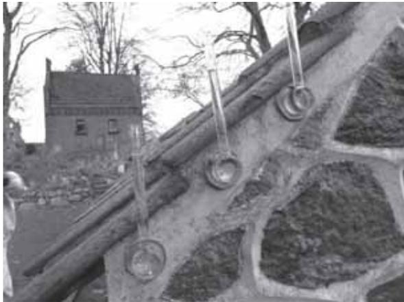
Figure 6. The 25% mortar developed by Ole Jensen was also used by the repair of a wall around the churchyard at Farum church. Picture is taken during measuring of capillarity with the Karsten tubes. (Photo: Martin Jensen)
