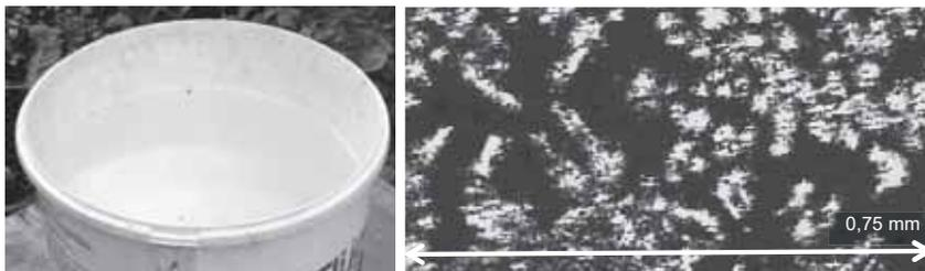
Figure 1. Carbonation on the surface of limewater. Crystals can be seen in the microscope.
