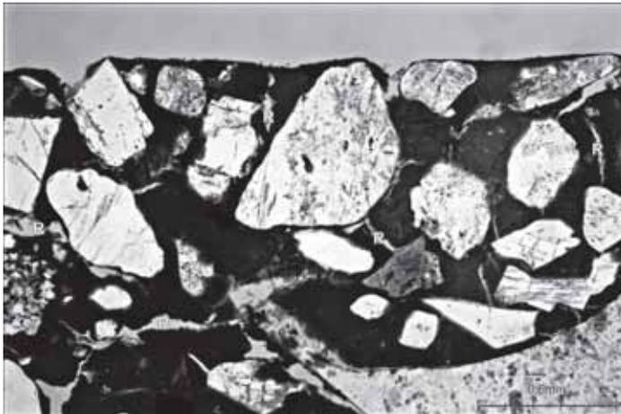
Figure 5. Enlargement of the section of the medieval mortar. The “R’s” show cracks.
