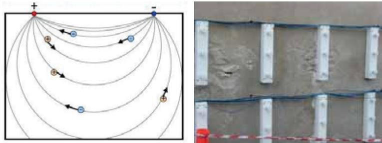
Figure 5: (a) principle of electro-desalination of wall with electrodes placed at the same side of the wall and distribution of electric field lines in case of a homogeneous material. (b) Photo from a pilot scale plant for electro-desalination of walls.
