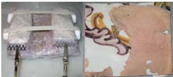
Figure 3: (a) Experimental setup for desalination of single tile; (b) 20<sup>th</sup> century tile used in lab experiment.
