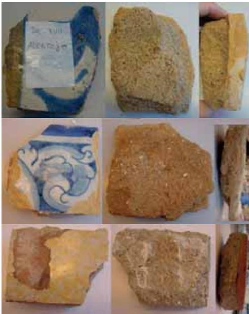
Figure 4: experimental tiles with mortar. Top: 17<sup>th</sup> century tile from Alentejo (PT); middle: 18<sup>th</sup> century tile from Palacio Centeno, Lisbon; bottom: 20<sup>th</sup> century tile of unknown origin.
