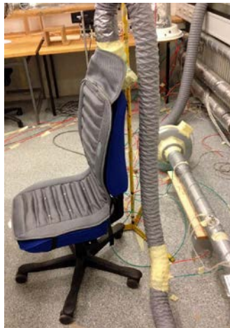
Figure 2. The ventilated cushion (VC) positioned on the computer chair and connected to the exhaust duct.
