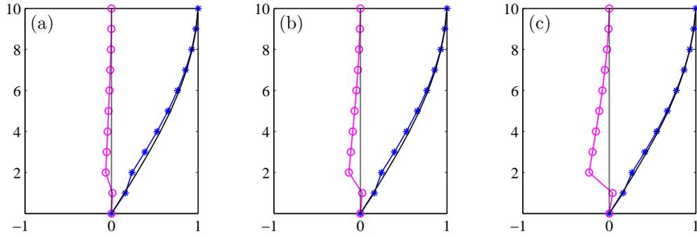
FIGURE 5. Real (blue  $*$ ) and imaginary (magenta  $\circ$ ) part of complex mode shape  $\mathbf{u}_1$  for the maximum modal damping case with  $\nu = 0$  (a),  $-2.0$  (b) and  $-4.0$  (c).
