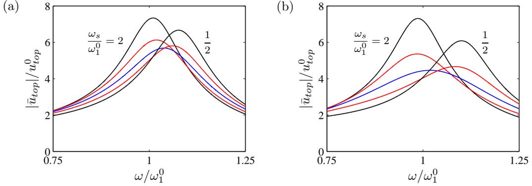
FIGURE 8. Top floor response with (a)  $\nu = -2.0$  and (b)  $-4.0$ , and  $\tau = \sqrt{1 - \nu/\omega_s}$  with  $\omega_s/\omega_1^0 = 2$  (black),  $\frac{4}{3}$  (red), 1 (blue),  $\frac{3}{4}$  (red) and  $\frac{1}{2}$  (black).
