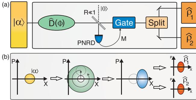
FIG. 1. (Color online) (a) Schematic of the cloning scheme. Two identical clones  $\hat{\rho}_{1,2}$  are created by probabilistic amplification and subsequent symmetric splitting. (b) Evolution of a coherent state in phase space during the cloning process.
