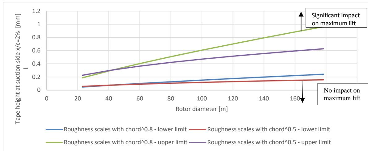
Figure 7 Bump/zigzag tape height on suction side at  $x/c=2\%$  and  $r/R=80.7\%$  as a function of rotor diameter. Curves show the lower and upper limit of roughness for influencing maximum lift. For both lower and upper limit trends following  $c^{0.5}$  and  $c^{0.8}$  are shown.
