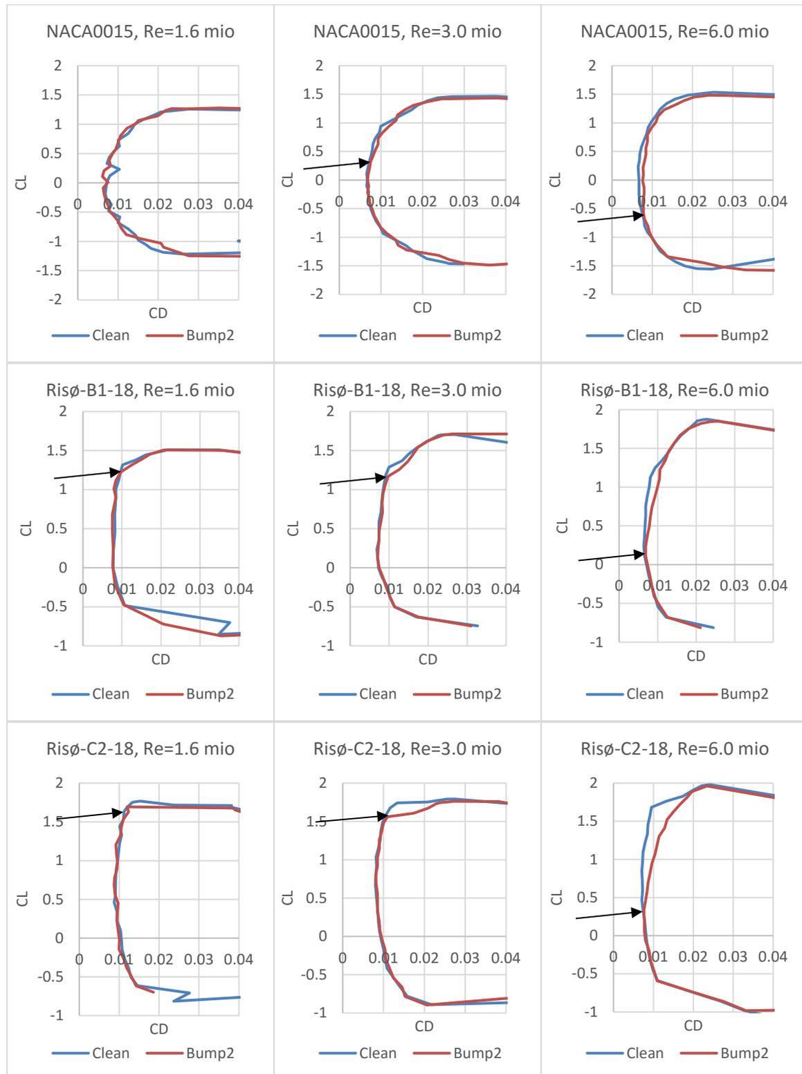
Figure 3 Lift coefficient  $c_l$  as a function of drag coefficient  $c_d$  for three different airfoils: 1) NACA0015 (top), 2) Risø-B1-18 (mid) and 3) Risø-C2-18 (bottom) and for three different  $Re$ : a)  $Re = 1.6 \times 10^6$  (left), b)  $Re = 3.0 \times 10^6$  (mid) and c)  $Re = 6 \times 10^6$  (right). The arrows indicate at which  $c_l$  the lift-drag ratio decreases caused by the LER.
