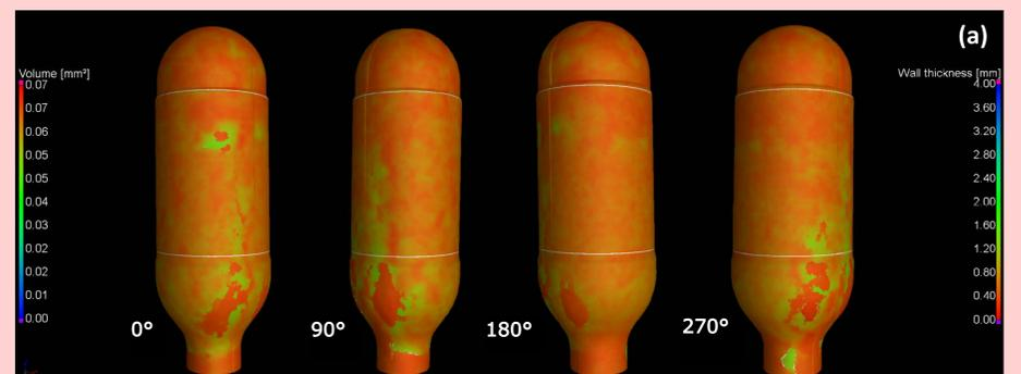
The insert used for fiber compaction is unable to compact pulp in the region of smooth curvatures due to which the neck region experiences higher wall thickness and low localized density.
