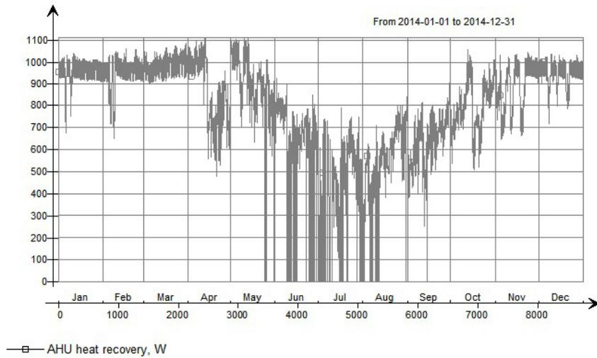
Fig. 3. Energy recovered in air handling unit.
