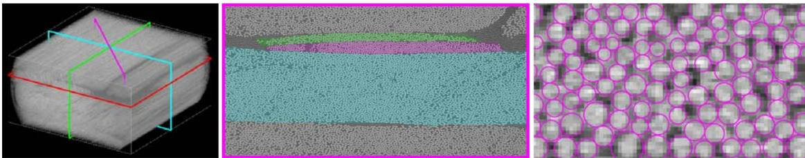
Figure 1: Cut planes for the bundle and fiber segmentation, a 45° bundle segmentation, and a close-up of a corresponding fiber segmentation. Cut planes, bundles and fibers are visualized in colors cyan: 0°, magenta: 45° and green: 90°
