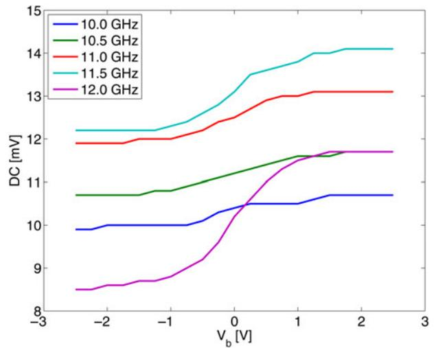
Fig. 13. DC level versus tuning voltage for different frequencies.
