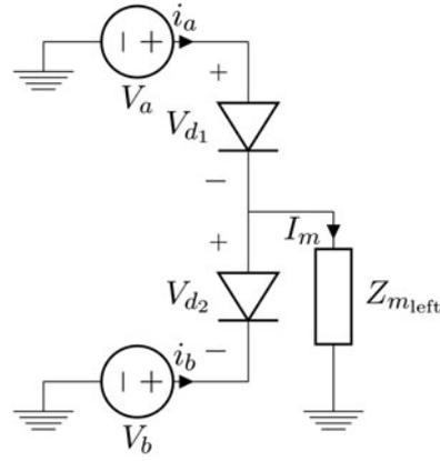
Fig. 16. Half circuit of diode ring, left side.
