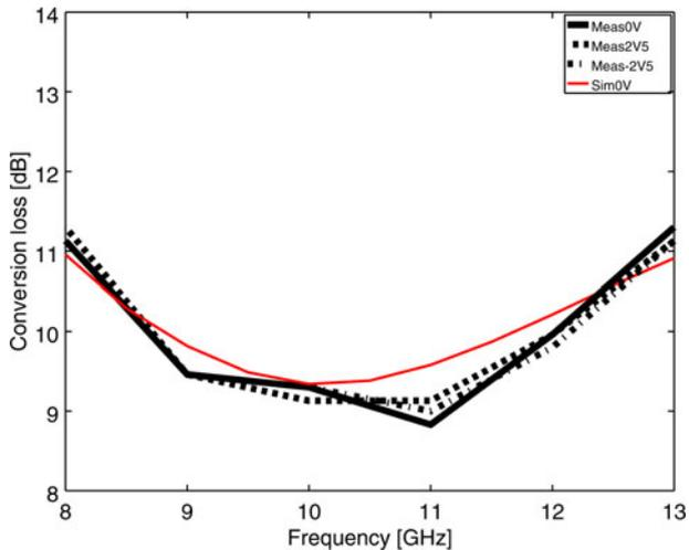
Fig. 11. Conversion loss as a function of frequency.
