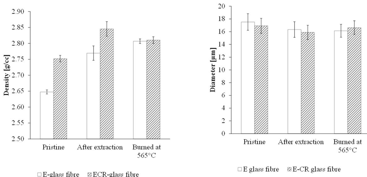
**Figure 1.** The densities of E-glass and ECR-glass fibres pristine and after removal of sizing by soxhlet extraction or burning at 565°C, all determined by use of a pycnometer.
