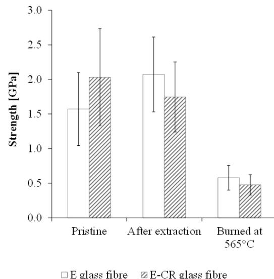
**Figure 4.** The strength of E-glass and ECR-glass fibres pristine and after removal of sizing by soxhlet extraction or burning at 565°C, obtained by single fibre tensile testing.
