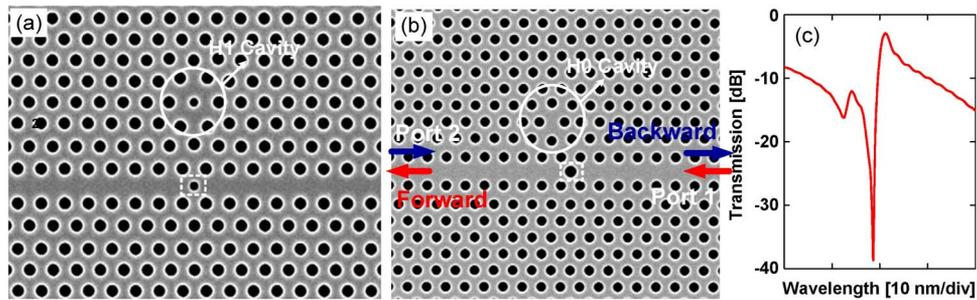
Fig. 3. (a) Fabricated InP membrane structure. (a) Symmetric Fano structure with an H1 nanocavity. (b) Fano structure with an H0 nanocavity is made asymmetric with respect to the mid-plane by displacing the blocking hole (BH) by one lattice constant towards port 1. (c) FDTD-simulated transmission spectrum of the asymmetric Fano structure.
