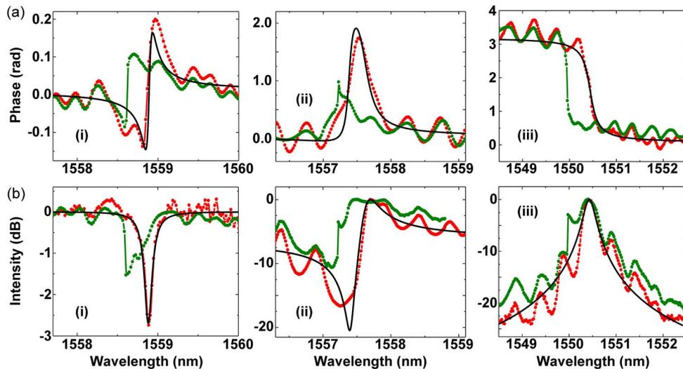
Fig. 4. Measured (a) phase and (b) intensity spectra of (i) open ( $t_B^2 = 1$ ), (ii) partially-blocked ( $t_B^2 = 0.1$ ), and (iii) blocked ( $t_B^2 = 0$ ) structures for two different input powers. Red and green dotted lines are experimental data at low and high input powers, respectively, and black solid lines represent theoretical fits to the low-power, linear case. All the structures have similar cavity Q-factors.
