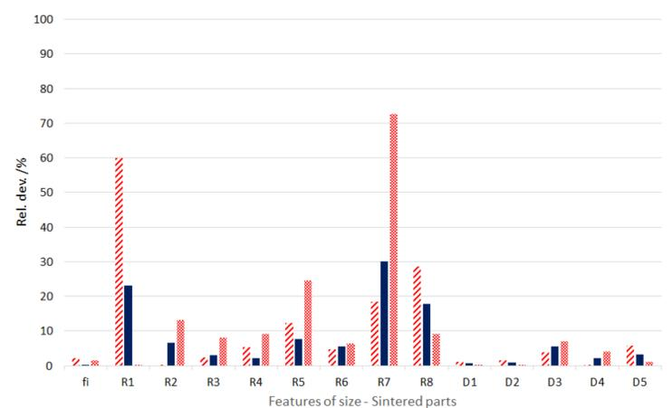
Figure 4. Relative deviations between the measurements of the sintered parts performed by OCMM and FVM. FVM is considered as reference. Considering the expanded uncertainty  $U$ , the red-dashed columns (▨) are the relative deviations between the lower limits  $d_{OCMM}-U$  and  $d_{FVM}-U$ ; while, the red-dotted columns (▩) are the relative deviations between the upper limits  $d_{OCMM}+U$  and  $d_{FVM}+U$ .
