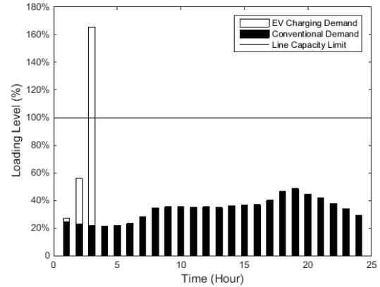
Fig. 6. Loading level of Line L23 without DLMP.
