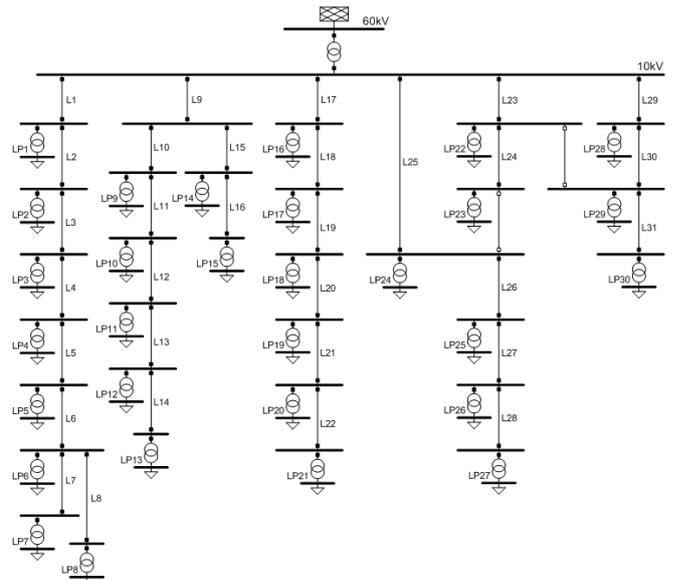
Fig. 2. Single line diagram of the distribution system for the case studies.
