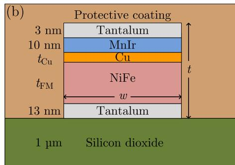
FIG. 1. (a) Illustration of the PHEB sensors with definitions of parameters and coordinate system. The grey and yellow colors indicate the sensor and contact stacks, respectively. (b) Illustration of the magnetic stack cross-section at the dashed line in (a).
