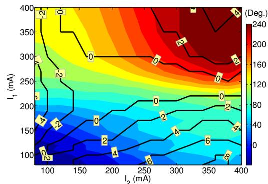
Fig. 5. Experimental demonstration of microwave phase shift (colour contour) and relative power change (black solid lines). The measurements are shown as a function of the currents  $I_1$  and  $I_2$  with  $I_3$  being fixed at 80 mA, and performed at 40 GHz.
