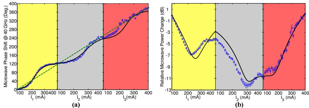
Fig. 4. Experimental demonstration of 360° microwave phase shift. (a) Microwave phase shift and (b) power changes at the microwave frequency of 40 GHz. The injection currents ( $I_1$ ,  $I_2$ ,  $I_3$ ) are increased from 80 mA to 400 mA consecutively. The markers are experimental data and the black solid lines are numerical simulations. The green dashed line shows a linear fit.
