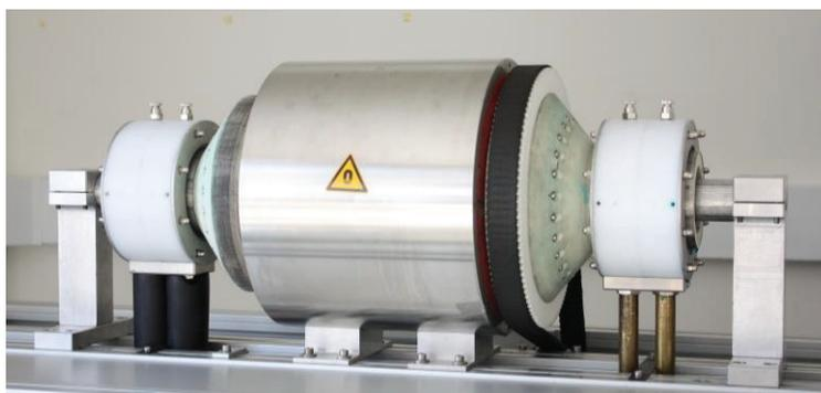
Figure 1. Rotating active magnetic refrigerator at DTU.
