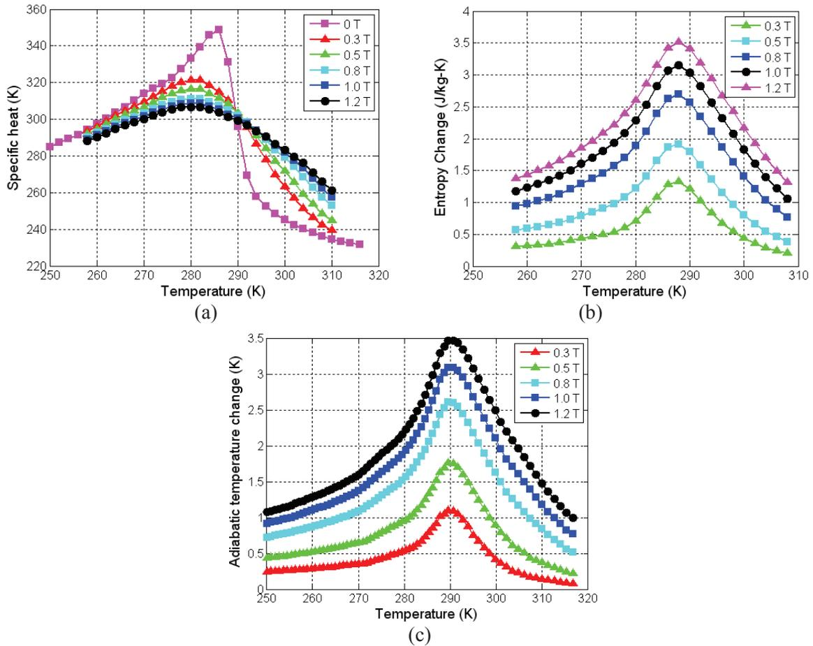
Figure 2. Properties of commercial Gd spheres used in the regenerator beds (a) Specific heat (zero-field is measured, the other curves are derived from  $\Delta s_{\text{mag}}$  from magnetization data and the zero-field specific heat) (b)  $\Delta s_{\text{mag}}$  integrated from the specific heat, and (c)  $\Delta T_{\text{ad}}$  as a function of temperature and magnetic field (derived from the specific heat and  $\Delta s_{\text{mag}}$  data).
