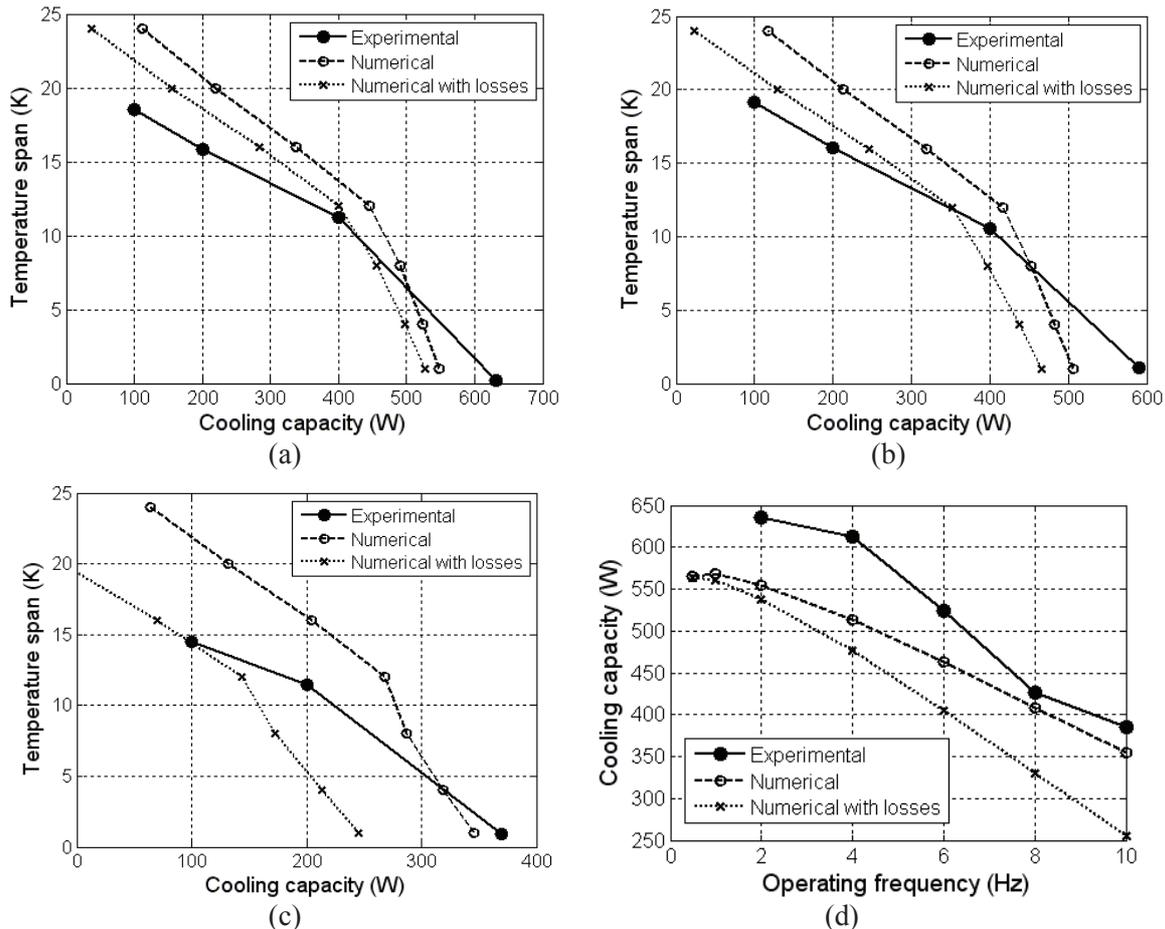
**Figure 5. Comparison of experimental and numerical results at (a) 2 Hz, (b) 4 Hz and (c) 10 Hz and (d) Maximum cooling capacity at no-span.**
