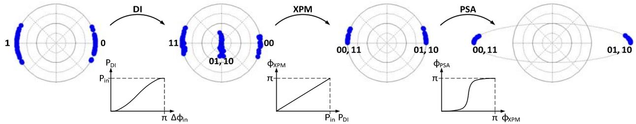
Fig. 2. The three steps of data processing; DI, XPM and PSA. The transfer function of each step (shown below each arrow) is applied to a PRBS with Gaussian phase noise. The DI converts phase modulation to modulation of output power by interfering two consecutive bits. XPM converts modulation of the signal power to phase modulation, either 0 or  $\pi$ , of the data carrier. Finally, the PSA regenerates the phase modulation by squeezing the phase.
