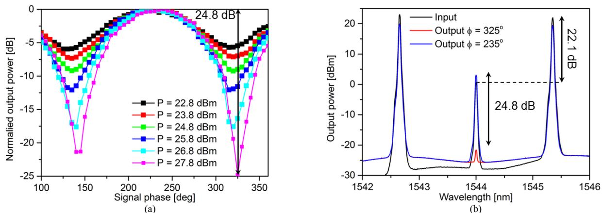
Fig. 6. Characterization of static operation of the PSA. (a) Normalized phase sensitive gain of the signal as a function of signal phase for increasing levels of total power  $P$ . (b) Spectra at the input and output of the HNLF-SPINE for maximum and minimum output signal power for a total input power of 27.8 dBm.
