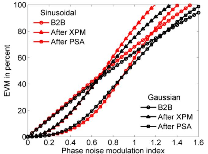
Fig. 10. Optical error-vector magnitude (EVM) as a function of modulation index  $m$  for sinusoidal (red) and Gaussian (black) input phase noise distributions, for the signal B2B (circle), after XPM (triangle) and at the output (square).
