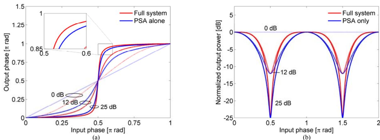
Fig. 3. Theoretical transfer functions for the data modulation in an ideal system, compared to that of an ideal PSA, for PSERs of 0 dB (dotted), 12 dB (dashed) and 25 dB (solid). ( $g = 1, 2.0$  and  $4.2$  respectively.). (a) Phase-to-phase and (b) phase-to-power.
