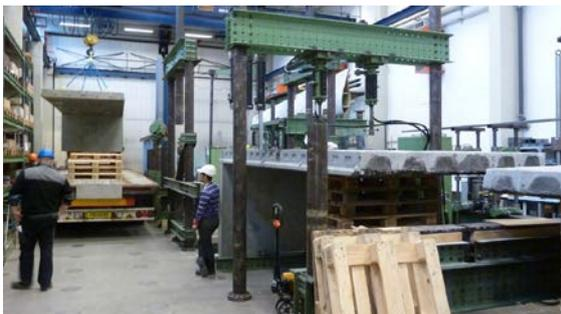
Fig. 18 Connected walls and decks at test rig.
