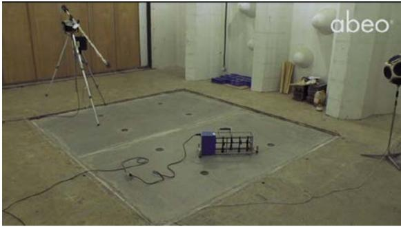
**Fig. 6** SL-Deck in accredited sound insulation and step noise test.
