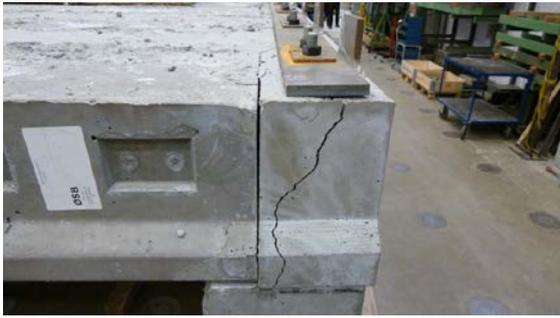
Fig. 20 Broken joint.
