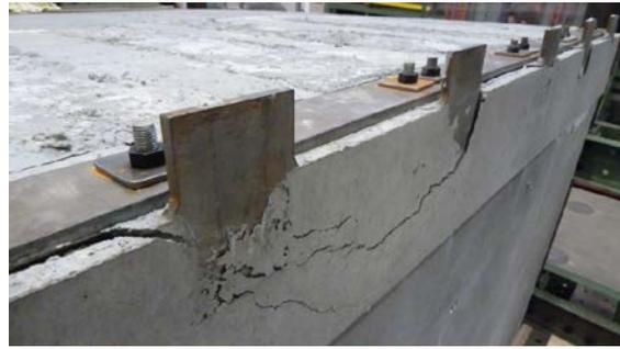
Fig. 21 Broken joint.
