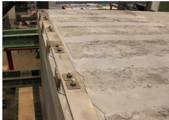
Fig. 23 Cracks at top of joint.
