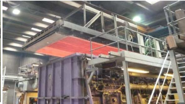
**Fig. 7** SL-Deck after 240 min accredited fire test.
