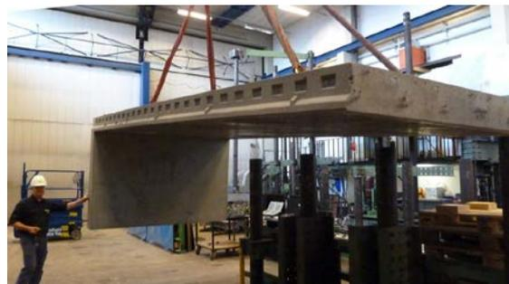
Fig. 19 Lifting of frame corner test specimen
